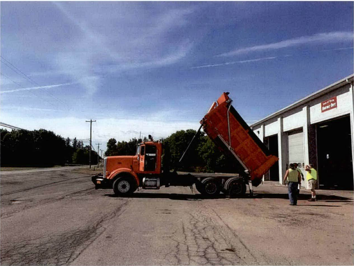
Measuring necessary height for the dump body when in raised position.
